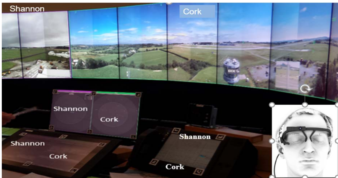
Figure 4.2. ATCO's Using Pupil Pro Eye Tracker interacted with RTM comprised OTW, RDP, EFS and VCS for Multiple Remote Tower Operations.
