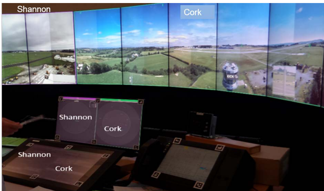
Figure 6.4 Controller Working Position (CWP) and Out of the Windows (OTW) screens of Remote Tower Module in RTC
