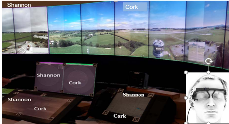
Figure 5.1. MRTO including infra cameras, pan tilt zoom and radar information for different airports shown by different colours on the boarder of displays: Green for Cork airport, Purple for Shannon airport
