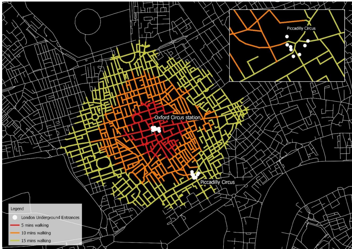
Figure 6-9 Service areas for 5, 10 and 15-minutes walking distance for Oxford Circus station only underground entrances/ exits.
