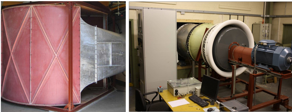
Figure 6.3: PWG test facility air chamber
