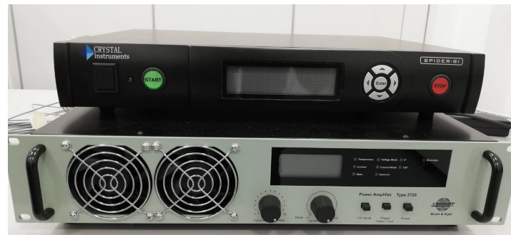
Figure G.4: Typical set-up of vibration control system (top) and power amplifier (bottom)
