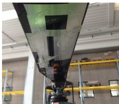
(a) FBGs mounted on rotor blade (reproduced from Serafini et al [8])
