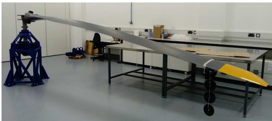
Figure 5.3: Typical structural loading test set-up
