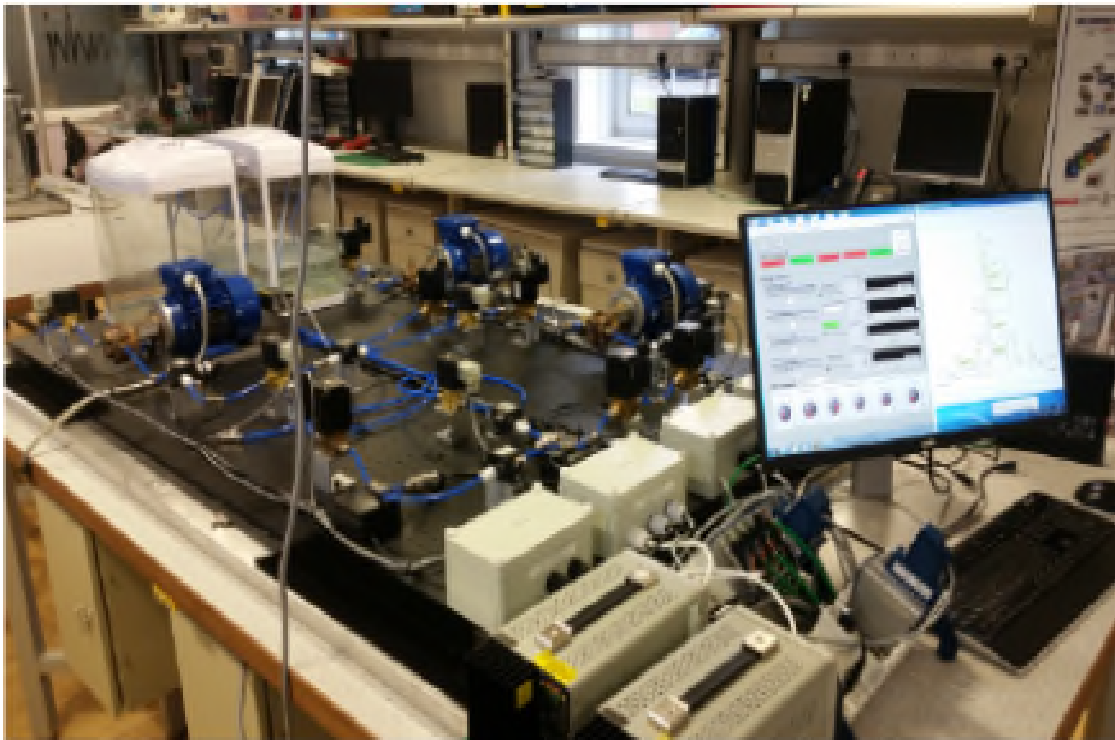
Figure 14 Aircraft fuel system test rig in Cranfield University IVHM Centre
