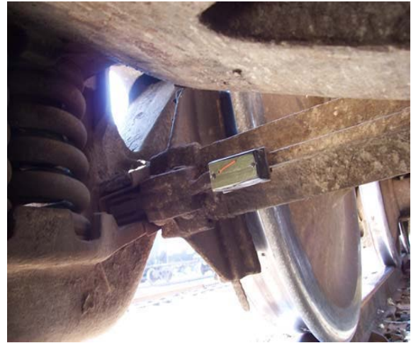
Fig. 5. Sensor mounted on a brake beam
