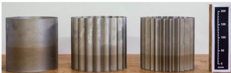
(a) Reference stainless steel circular shell and optimized, Aster and wavy shells 3D printed by powder bed fusion (reprinting permission for these images has been obtained from the publisher [157]).
