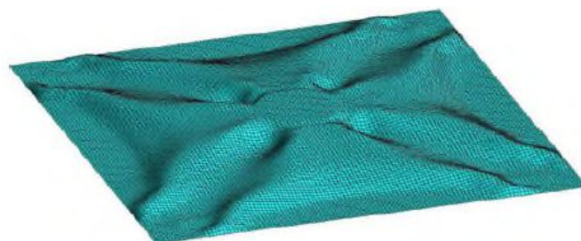
(b) Shape optimisation of a sheet subject to out-of-plane loads (reprinting permission for these images has been obtained from the publisher [158]).
