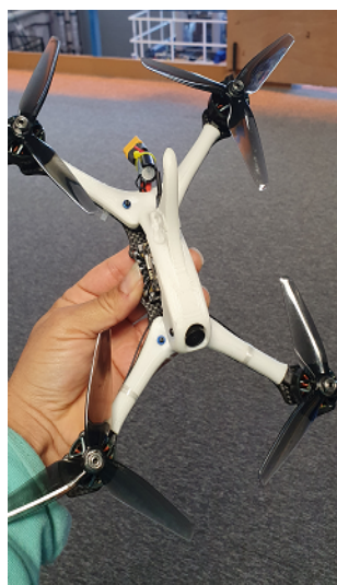
Figure 7: Non-Symmetrical Structure - NSY.
