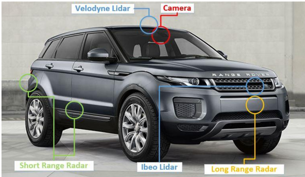
App.Figure A-5 The Advanced Version of sensors installation.
