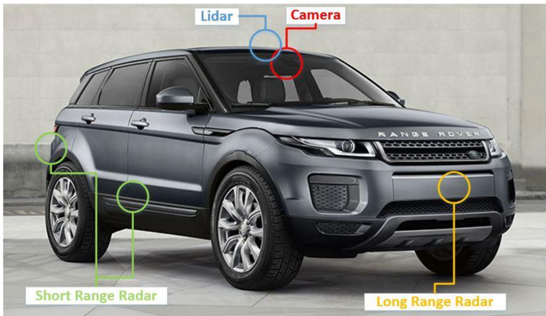
App.Figure A-3 The Medium Version of sensors installation.
