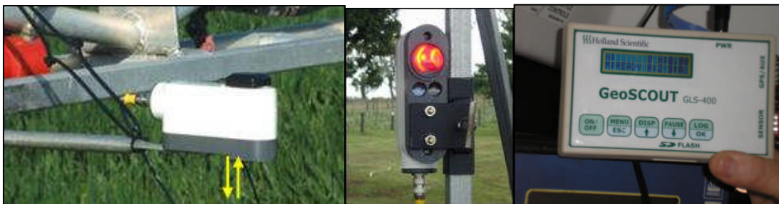
Figure 2-19 Crop Circle sensor and the GeoSCOUT logger
