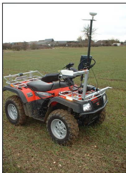
Figure 3-9 Crop Circle sensor mounted on Quad bike
