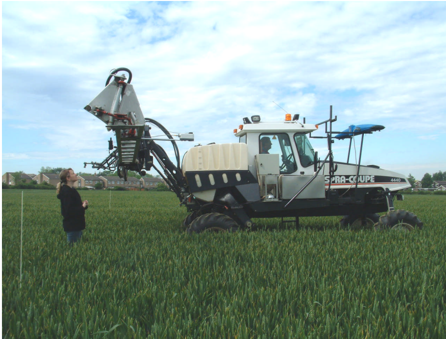
Figure 3-8 Scanning at site when using the Crop Circle mounted on the boom
