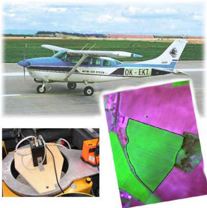
Figure 2-14 Aerial system Nitrosensing (MJM Litovel, 2007)
