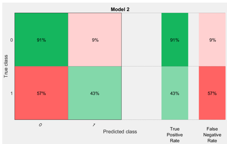
Figure 5-9: Confusion matrix showing True positive rate and False negative rate for Gaussian SVM model on German credit data (Class 0: Creditworthy, Class 1: Non-creditworthy).
