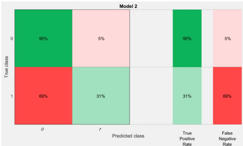
Figure 5-40: Confusion matrix percentage for KNN classifier on Taiwan credit data (Class 0: Creditworthy, Class 1: Non-creditworthy).
