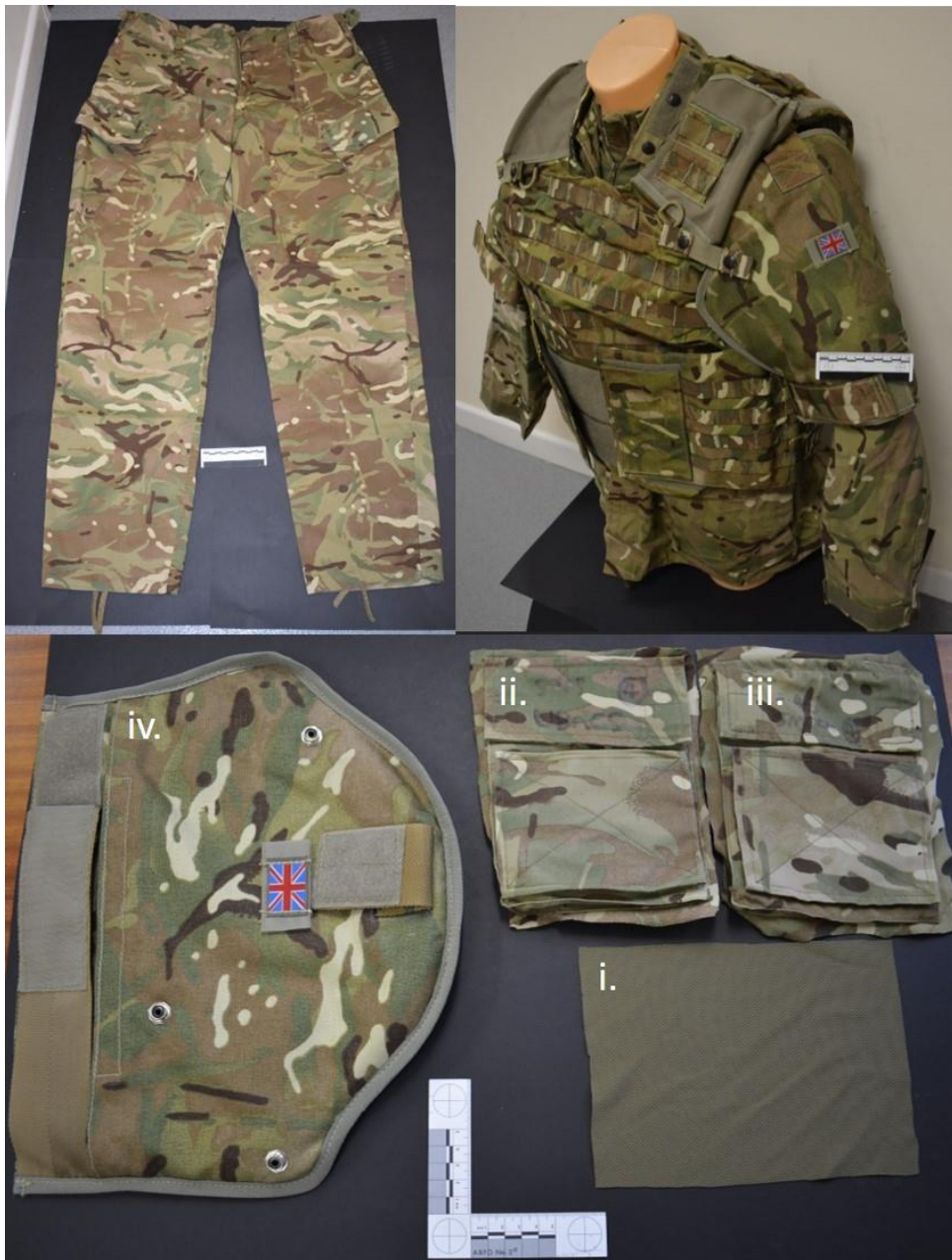
Figure 6.2 Examples of MTP clothing used – clockwise from top left: MTP trousers; top right: t-shirt, UBACS, smock, and brassard as worn by service personnel; bottom: i. t-shirt, ii. UBACS, iii. smock and iv. brassard layers prepared for testing. Laundering detail and fabric analysis data for this clothing used within these experiments is detailed in previously published work [9]
