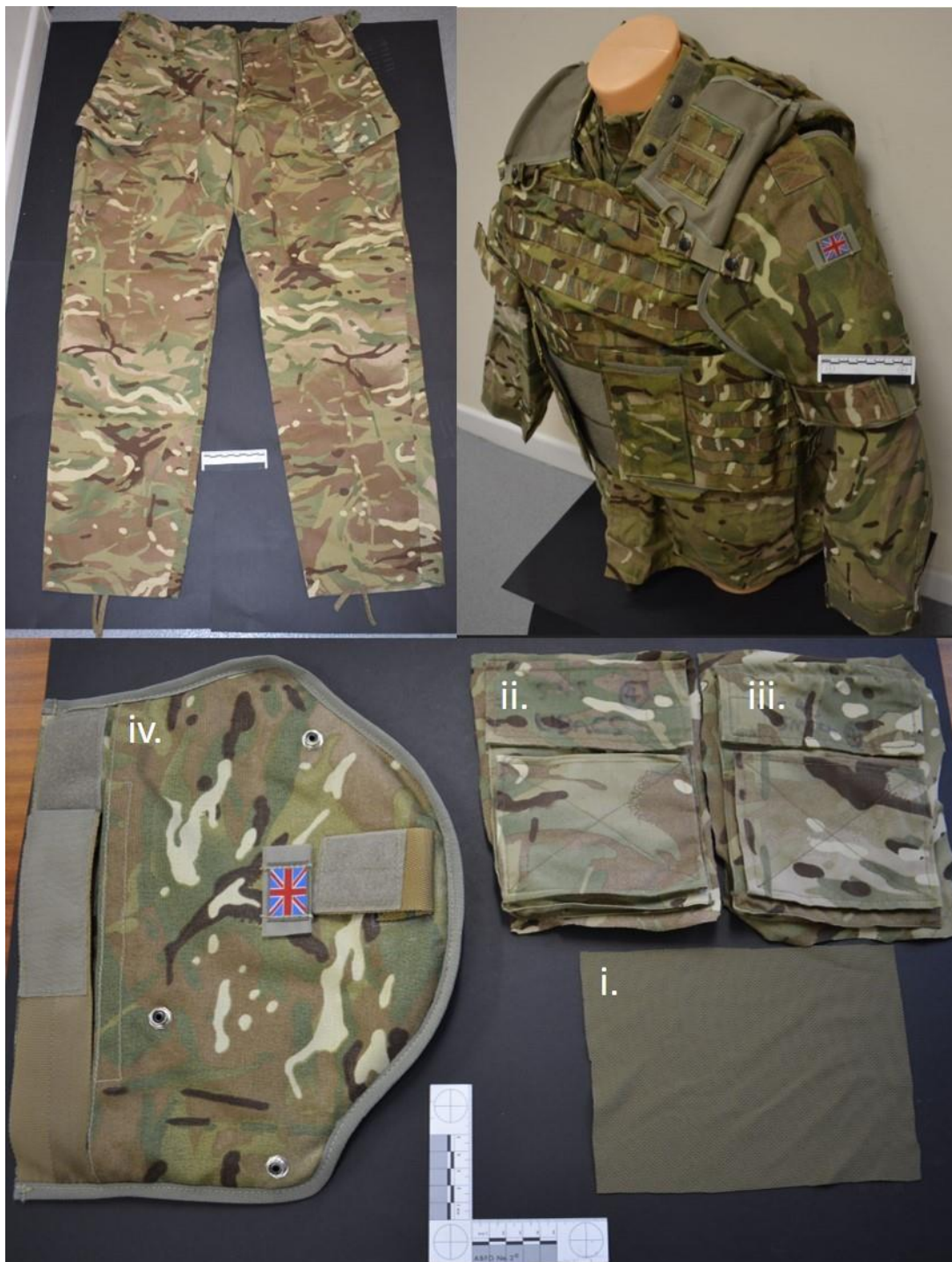
Figure 3.1 Examples of MTP clothing used – clockwise from top left: MTP trousers; top right: t-shirt, UBACS, smock, and brassard as worn by service personnel; bottom: i. t-shirt, ii. UBACS, iii. smock and iv. brassard layers prepared for testing
