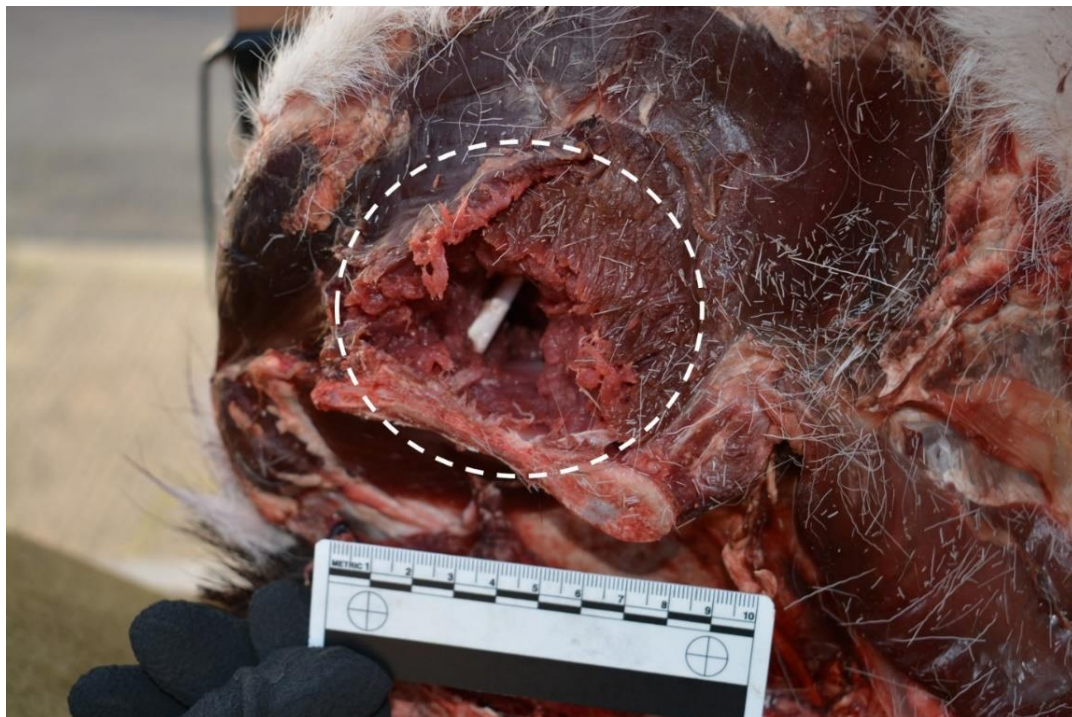
Figure 4.6 Example of large exit wound seen following yawing projectile exit the deer limb, indicated by dotted circle
