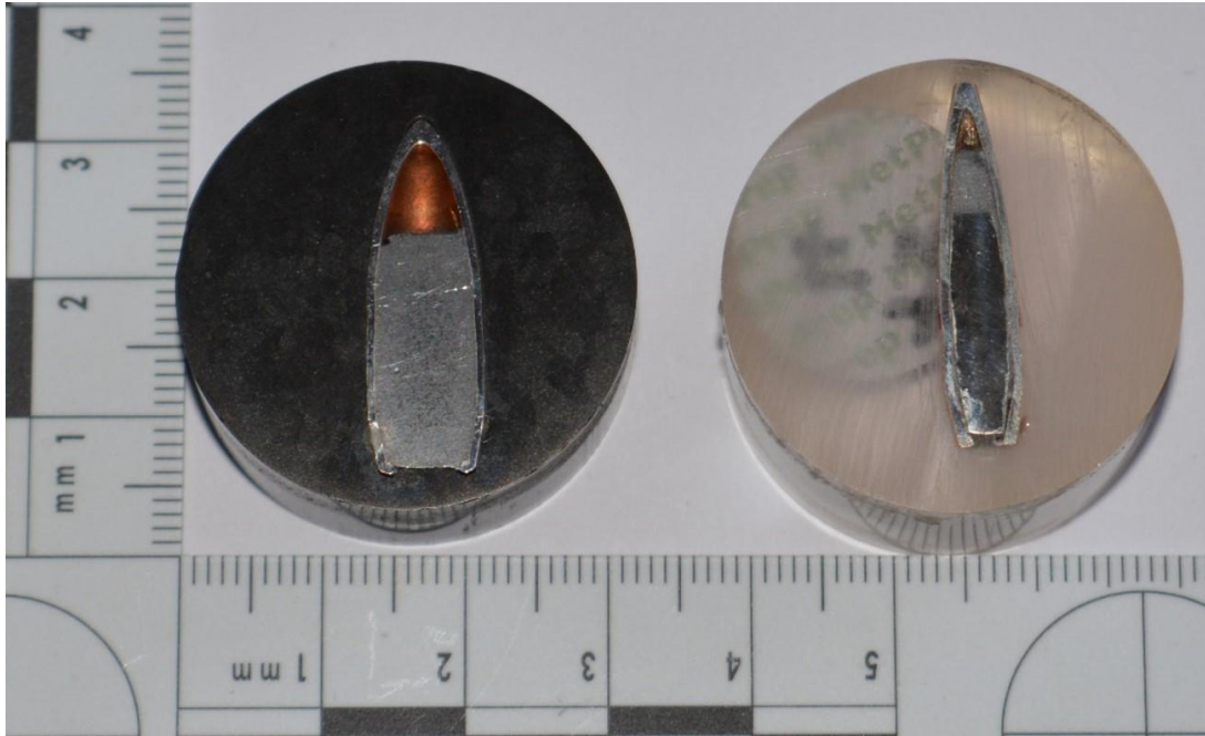
Figure 3.2 Mounted sections of 7.62mm (left) and 5.45mm (right) projectiles
