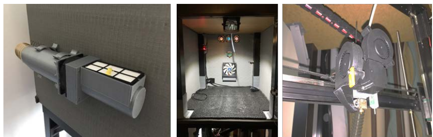
Figure 1. Final design dual extrusion system with radial fans.
