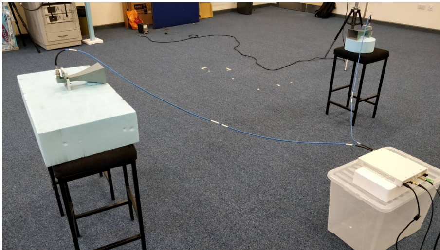
Figure 6.2: Photo of the experimental RF link for stationary channel isolation measurements.
