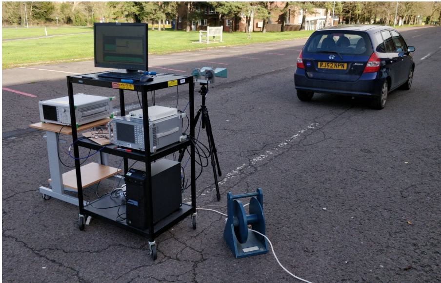
Figure 6.24: Photo of the experimental setup using MBR and a moving target.
