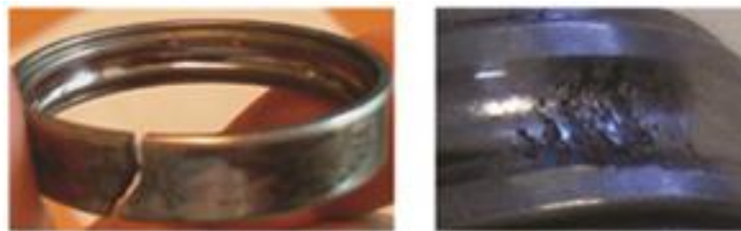
Figure 2-6 Bearing external ring failure and inner ring failure with fracture (Source: (Medjaher et al , 2012)) (see appendix A for permission)
