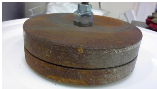
Figure 2-5 Metal discs showing corrosion on the surface
