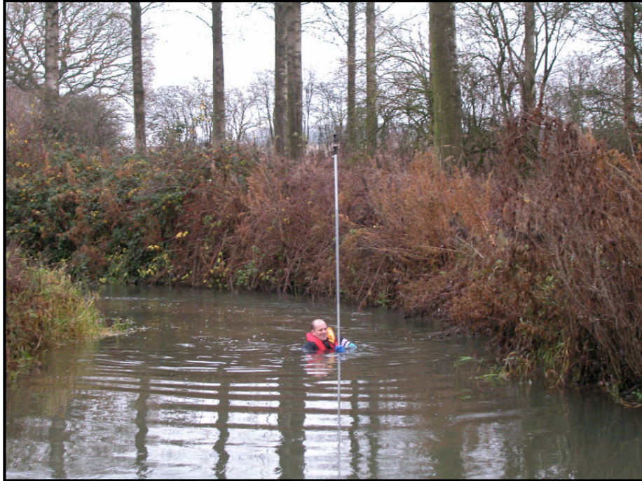
Figure 3.3: difficulties when measuring depth with the total station at deep points. The metric staff cannot be placed at deepest points because the data collector cannot walk any further (Windrush river site).
