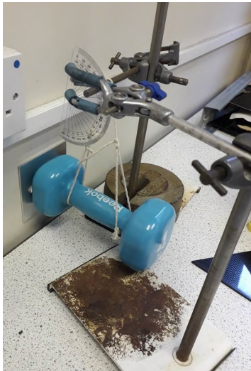
Figure 9 Experimental set up, showing 4 kg mass, aluminium plate and protractor.
