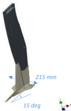
Figure 4.16. Sumo Trio working tine left: in the soil bin experiments; right: computer-aided design (CAD) showing its geometry
