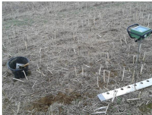
Figure 3.23. Penetrometer reading at field site
