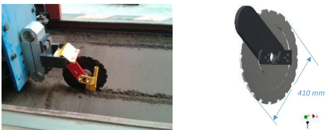
Figure 4.10. Väderstad Rapid's working disc left: in the soil bin experiments; right: computer-aided design (CAD) showing its geometry
