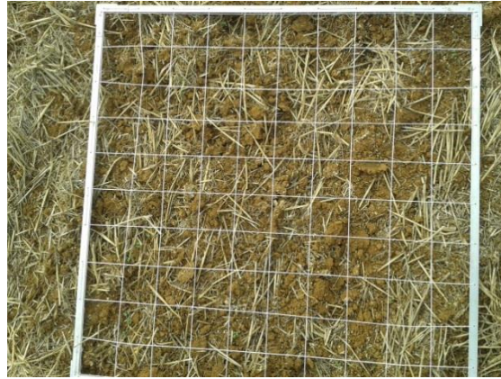
Figure 3.30. Surface residue measurements with a 1 m 2 quadrat
