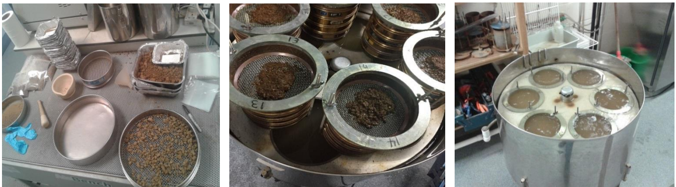
Figure 3.26. Soil preparation (left), samples prior to wet sieving (middle) and wet sieving (right)
