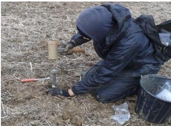
Figure 3.22. Sampling (left) and lab analysis (right) for bulk density
