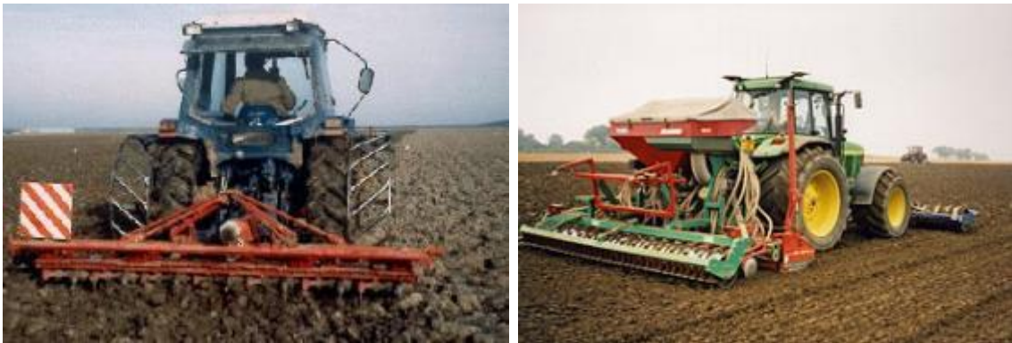
Figure 2.1. a) Seedbed preparation alone (left) and b) seedbed preparation and drilling in one pass (right)
