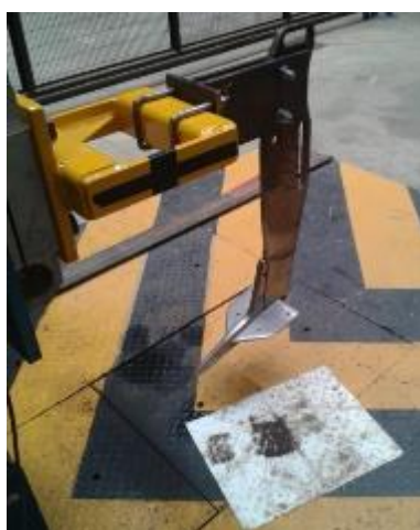
Figure 4.16. Sumo Trio working tine left: in the soil bin experiments; right: computer-aided design (CAD) showing its geometry
