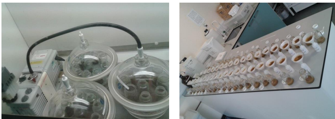
Figure 3.25. Fumigation (left) and organic carbon extraction in separate plastic bottles (right)
