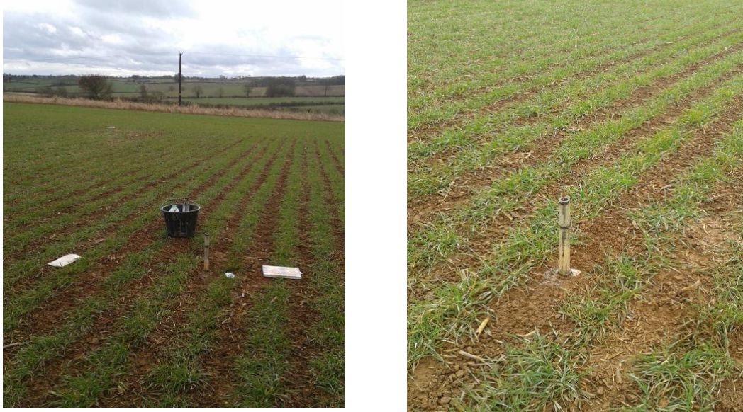
Figure 3.29. Unsaturated hydraulic conductivity measurements with the mini disk infiltrometer
