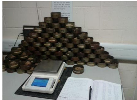
Figure 3.22. Sampling (left) and lab analysis (right) for bulk density
