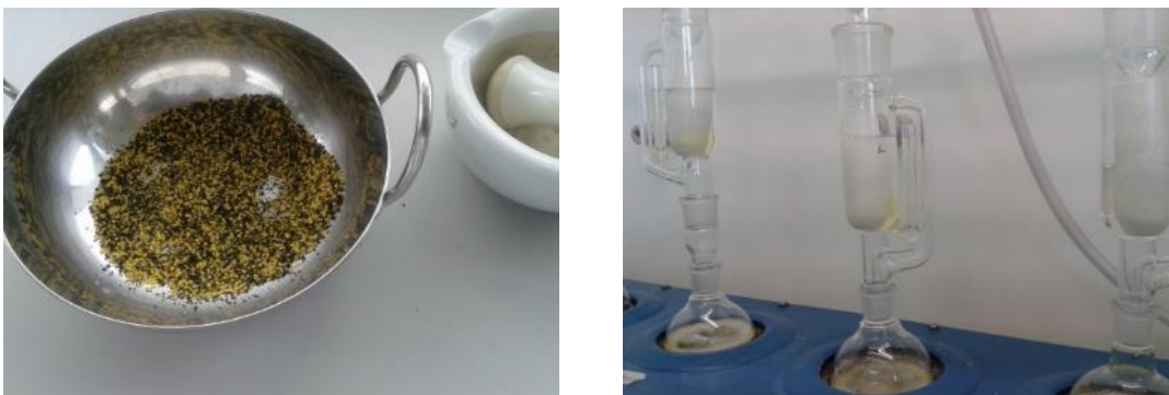
Figure 3.32. Ground seeds (left) and oil extraction with hexane solvent (right)
