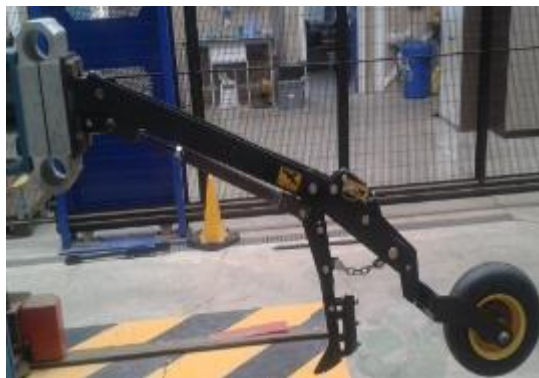
Figure 4.7. Väderstad Seed Hawk main working tine; left: in the soil bin experiments; right: computer-aided design (CAD) showing its geometry
