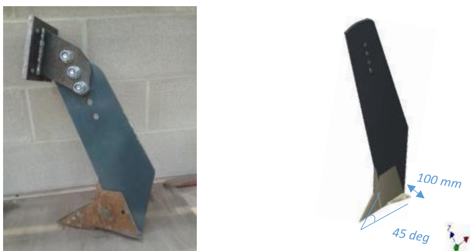
Figure 4.14. Mzuri's working tine left: in the soil bin experiments; right: computer-aided design (CAD) showing its geometry
