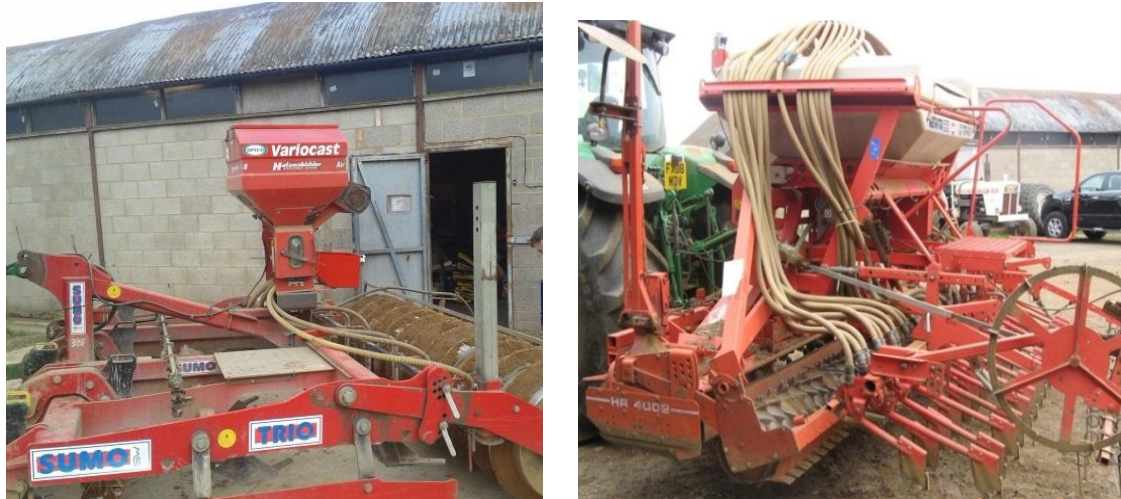
Figure 3.6. The farm system - Sumo Trio (used only in rape with the seed hopper; left) and Kuhn HR 4002 (plus Sumo Trio without the use of seed hopper used in wheat; right)
