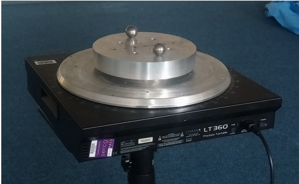
Figure A.5: Turntable and support plate. Two small spheres are fixed into a grooves directly on the support plate
