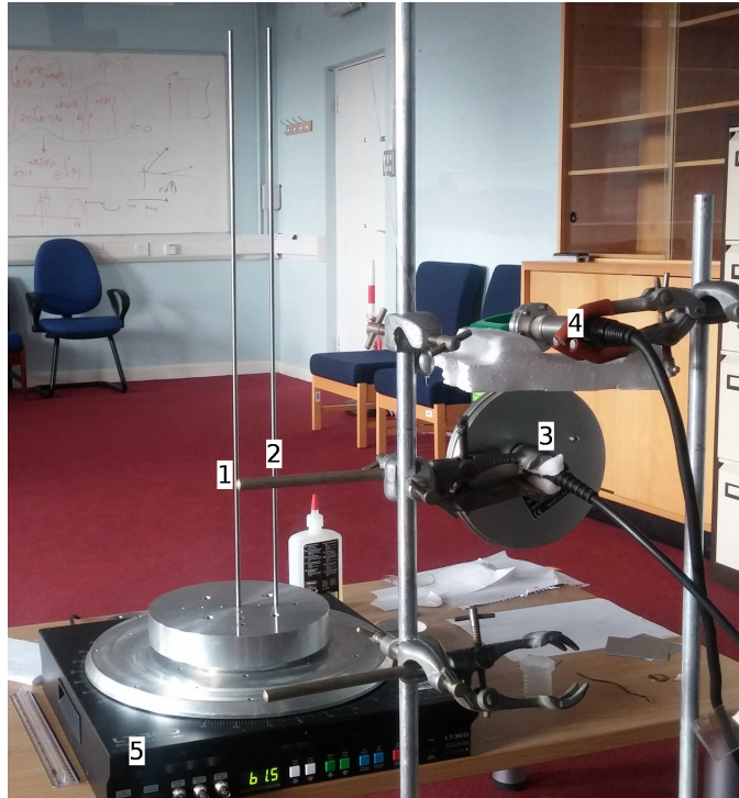
Figure 5.1: Ultrasound experimental set up – two vertical rods on a turntable: 1 – central rod; 2 – peripheral rod; 3 – ultrasound speaker; 4 – ultrasound microphone; 5 – turntable
