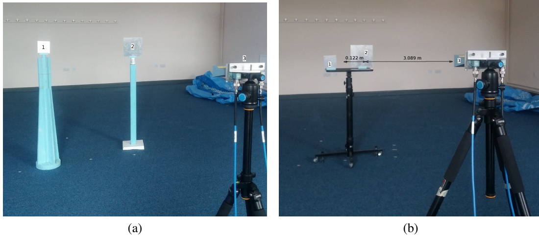
Figure 6.2: Two flat plates as a target: front plate – 1; rear plate – 2; radar antennas – 3
