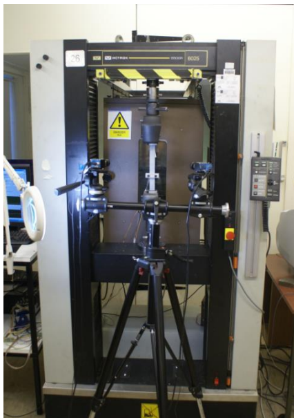
Figure 50: Load frame and digital cameras used for DIC
