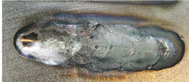
Figure 7.11 – Example of typical plasma weld surface condition.
