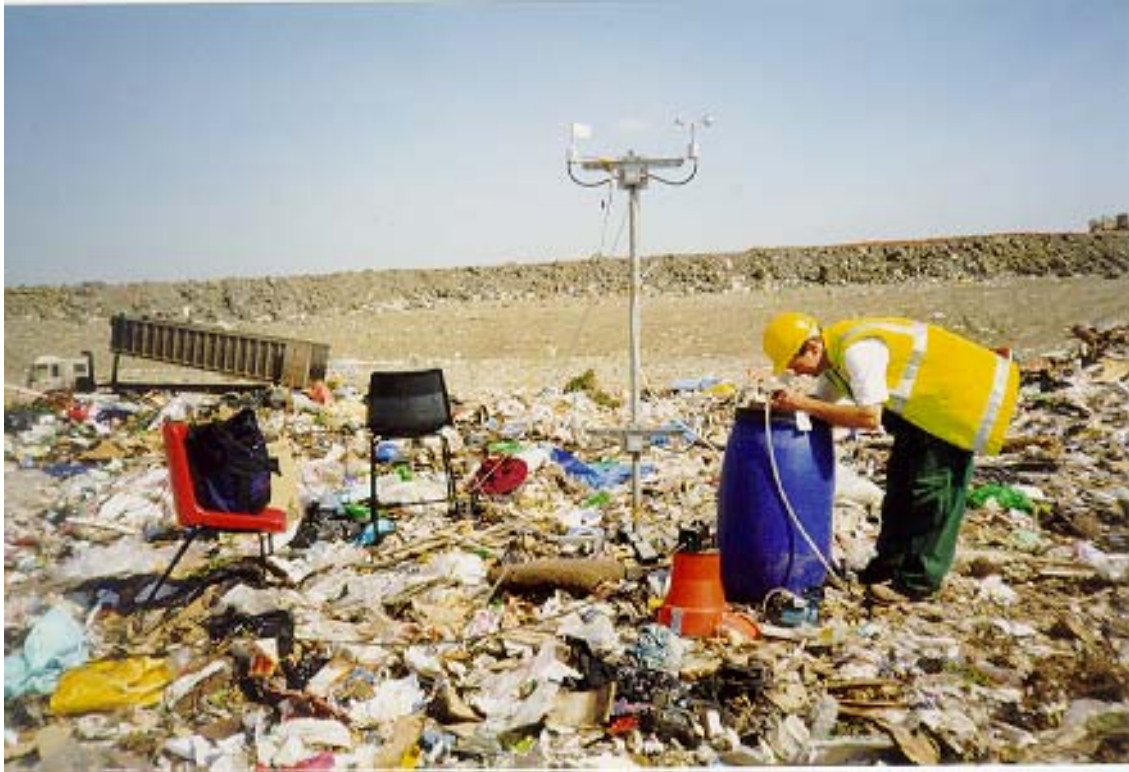
Figure 3.8 A distant view of the portable meteorological mast in use at the MSW Landfill Site with two sets of cup and vane anemometers, two sets of temperature and humidity sensors and a connection for the odour sampling. Date: 18 th August, 1998.
