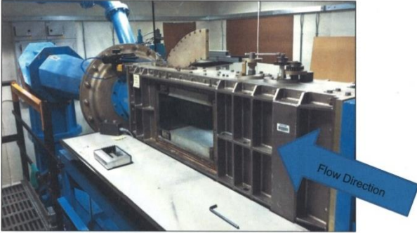
Figure 2. Transonic wind tunnel with side door removed
