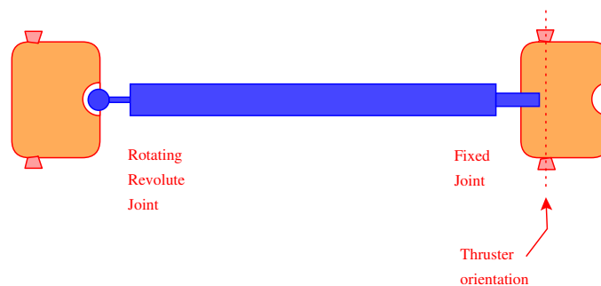
Figure 7.15: Attachment of links to microcells. Links are free to rotate at one end, and fixed the microcell at the other. This maintains an overall revolute joint at each microcell from a kinematic point of view, whilst allowing the thrusters of the cell to be correctly oriented.
