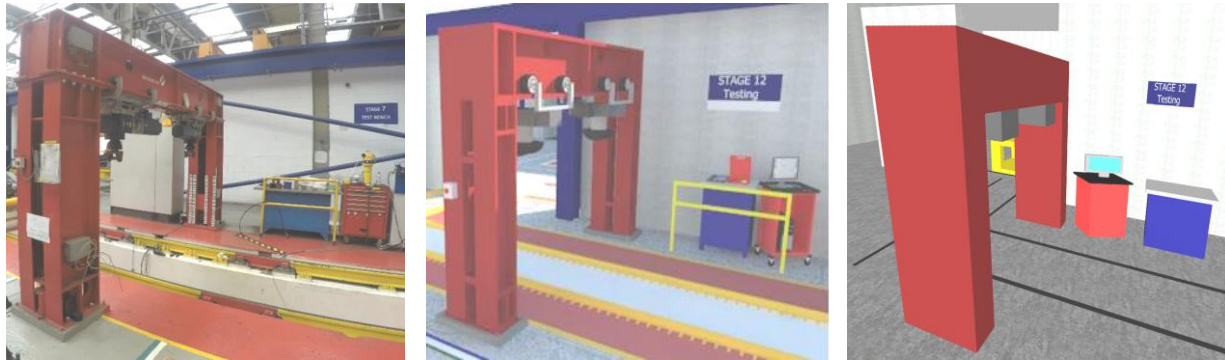
Figure 5: Actual shop floor and its immersive 3D models in high fidelity (middle) and low fidelity (right) (Petti et al. 2016) implemented in WITNESS 14 and viewed through Visionary Render.
