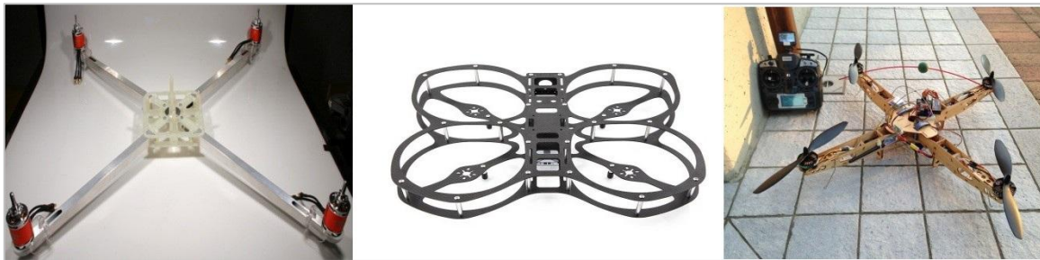
Figure 3-1: Type of frame. (left to right). Aluminium, Carbon Fibre, Plywood. (Multipilot 2011)
