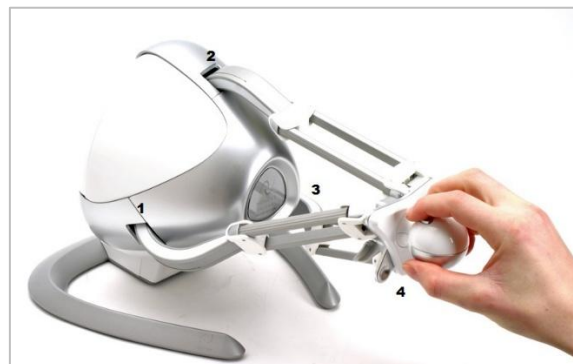
Figure 4-6: Novint Falcon haptic controller with multiple link (1-4) to motors for force feedback (Falcon 2014)
