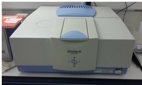
Figure 2.3 Shimadzu IRPrestige-21 Fourier transform infrared spectrophotometer
