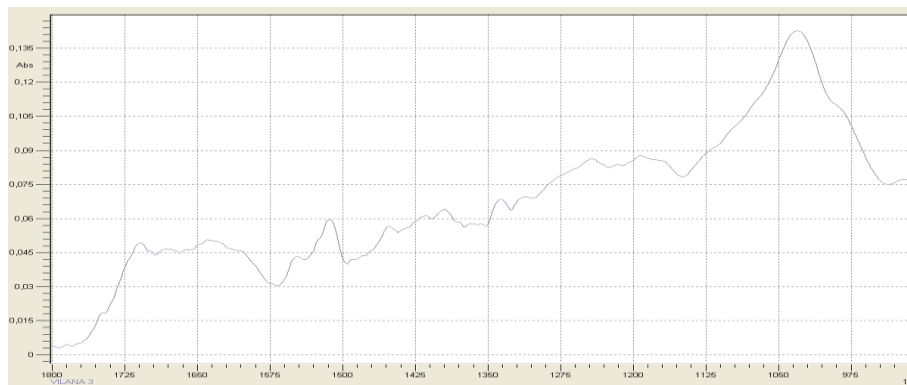
Figure A76: Absorption spectra of Vilana after 12 months of ageing in American oak barrel
