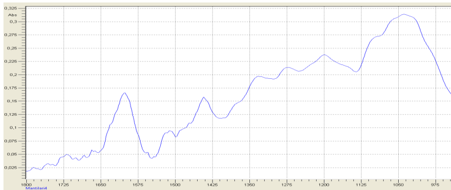
Figure A44: Absorption spectra of Mandilari after 6 months of ageing in acacia barrel
