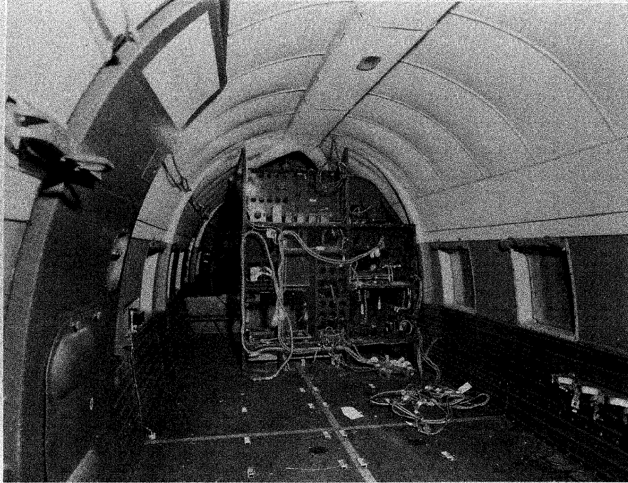
FIG. 4. REAR CABIN -- CREW SEATS REMOVED
