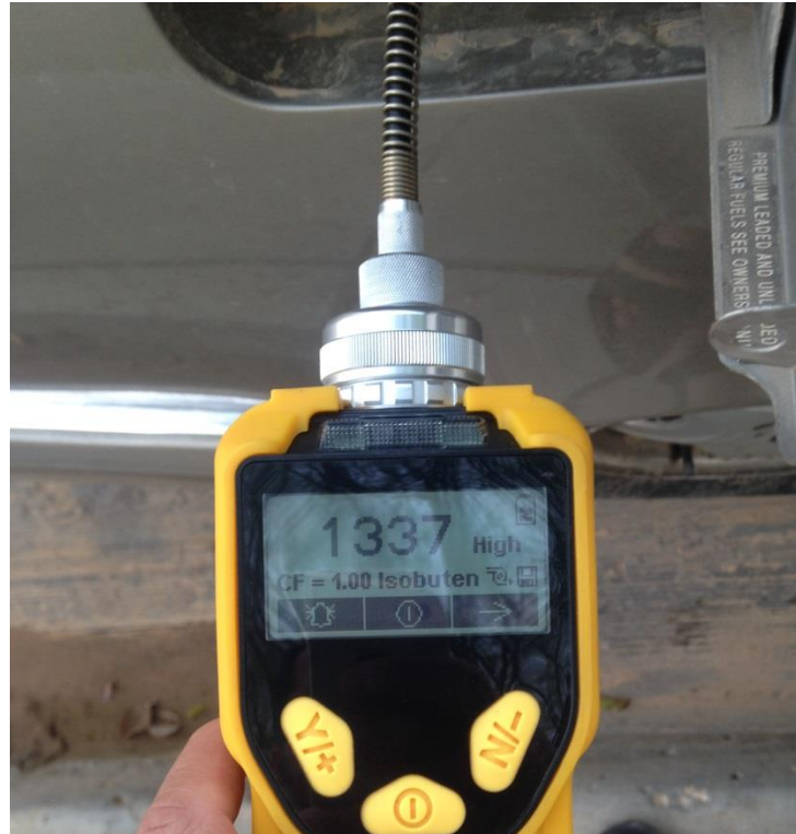
Figure 4-2: Direct reading measurement of gasoline vapour at vehicle fuel tank opening
