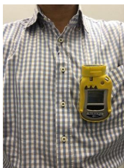
Figure 7-2: ToxiRae Pro PID personal VOC exposure monitoring instrumentation (Courtesy: Rae Corporation)
