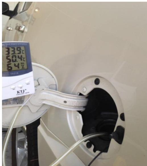
Figure 3-1: A modified dual sensor digital thermometer used to measure the gasoline temperatures inside and outside vehicle tanks and underground storage tanks
