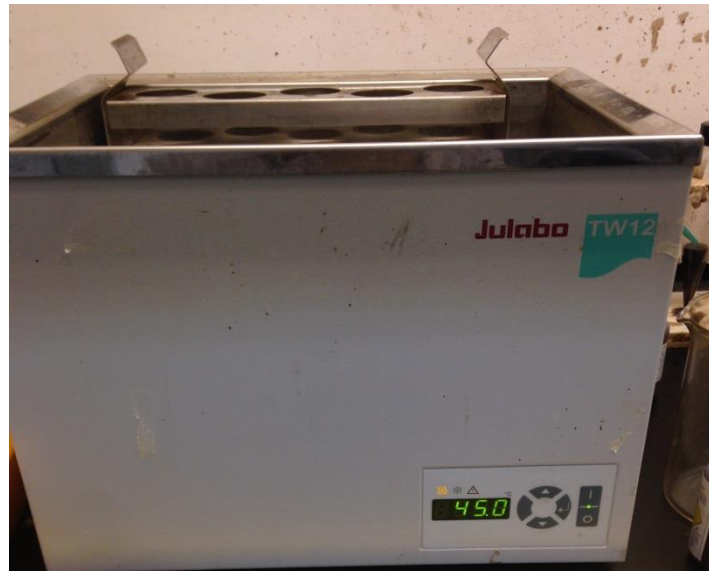
Figure 3-2 Heated water bath with temperature digital indicator for heating gasoline in vials.
