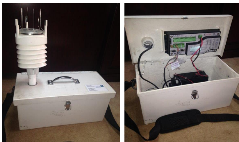
Figure 4-1: Portable mini-weather station designed and used in these studies
