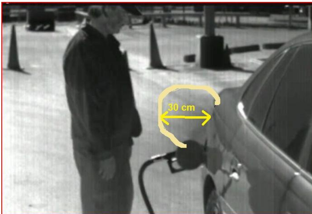
Figure 4-7: FLIR qualitative image illustrating gasoline vapour plume distance
