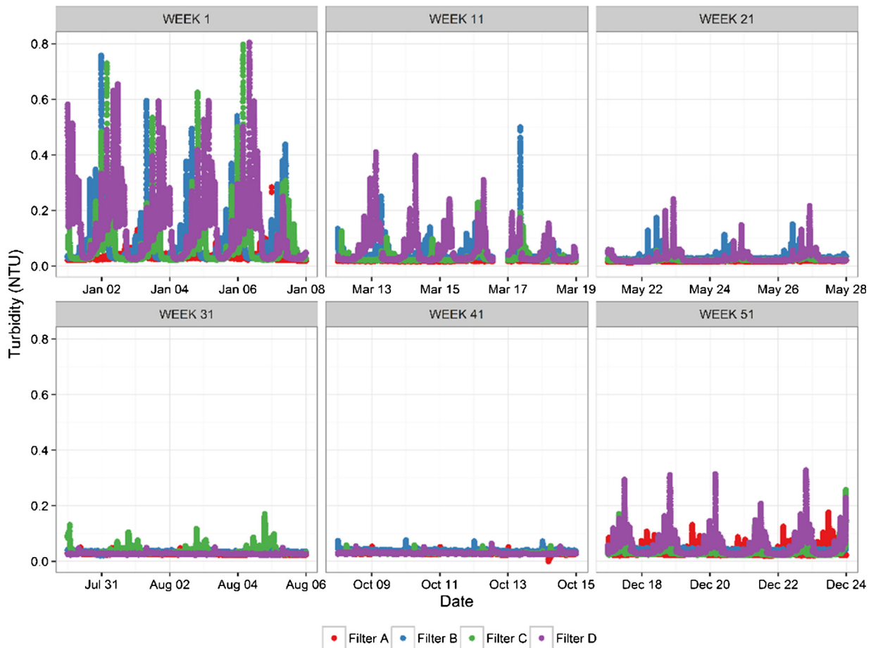
Fig. 2. Turbidity time series for weeks selected to demonstrate variation in filter performance.
