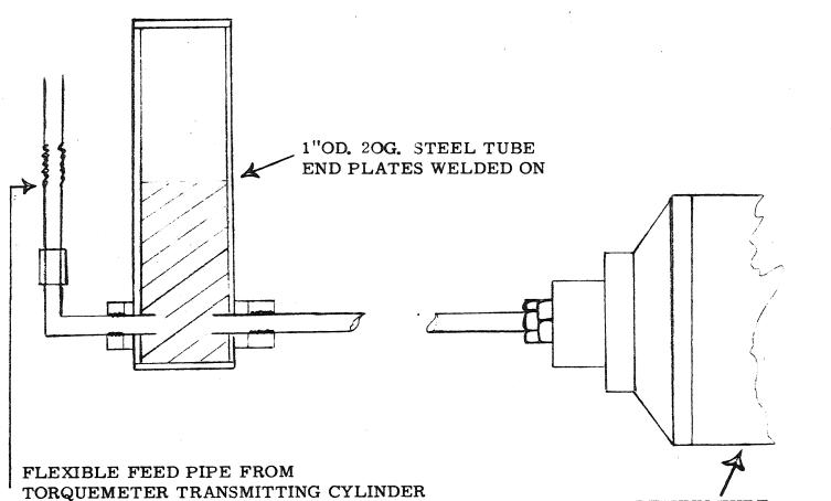
DESYNN TYPE OIL PRESSURE TRANSMITTER
