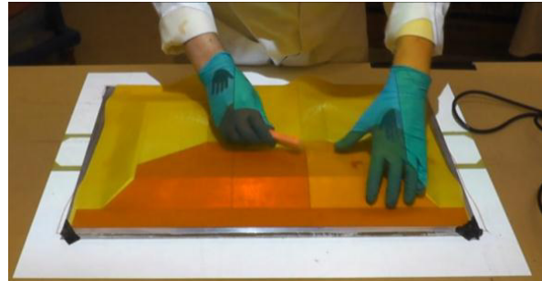
Fig. 13. Best case layup scenario - plain woven glass prepreg.
