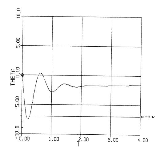
FIGURE A-4: PITCH RATE IMPULSE RESPONSE TO 1 DEGREE OF ELEVATOR.
