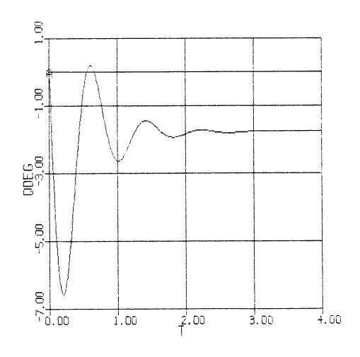
FIGURE A-3: PITCH ANGLE IMPULSE RESPONSE TO 1 DEGREE OF ELEVATOR.
