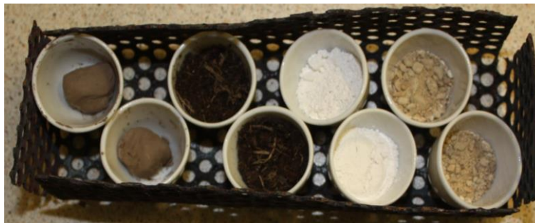
Figure 4-15: Crucibles containing control soils after 24 hours at 105°C
