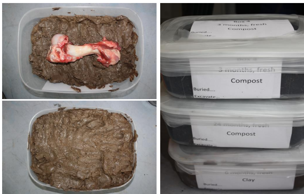
Figure 4-14: Photographs depicting porcine burial methodology of the porcine bones, in plastic boxes filled with the chosen medium, sealed with parafilm and labelled with burial/excavation date and burial medium
