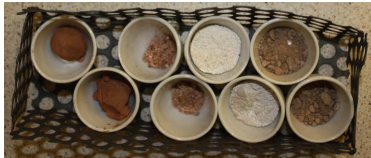
Figure 4-16: Crucibles containing control 'ashed' soils after 24 hours at 440°C
