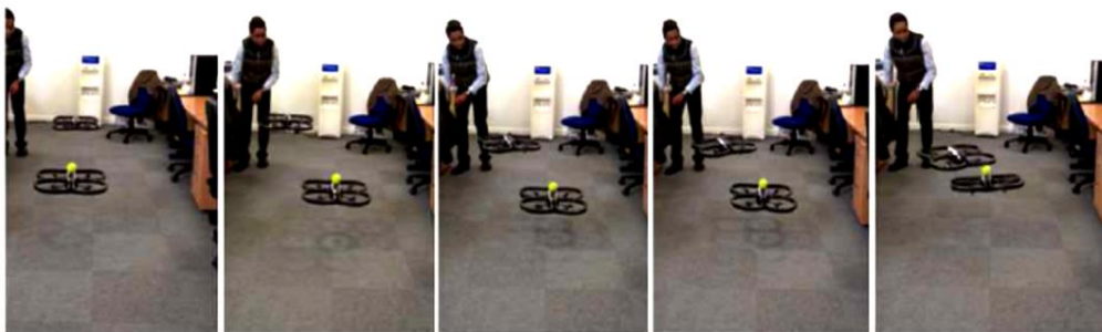
Figure 11. The first autonomous aerial flocking attempt with a stationary Leader micro-UAV and moving Follower micro-UAV did not result in continuous flocking of two vehicles.
