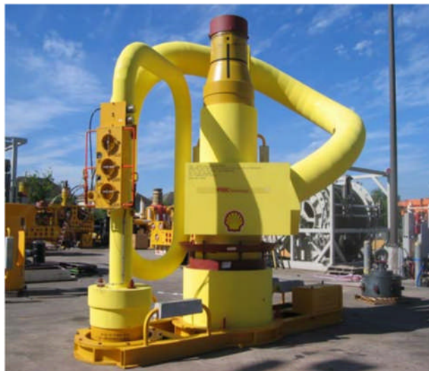
Figure 2-9 Photo including the inlet part of the Caisson separator used in the Perdido project (Vu et al. , 2008)
