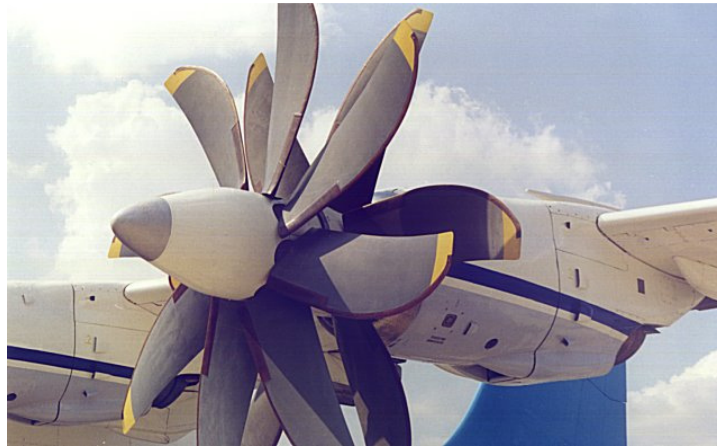
Figure 2-18 Ivchenko Progress D-27 contra-rotating propfan on Antonov AN-70 [25].
