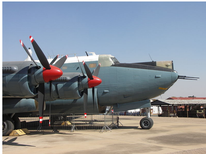
Figure 2-13 Avro Shackleton with Rolls Royce Griffon engines on display in S.A.A.F Museum [10].
