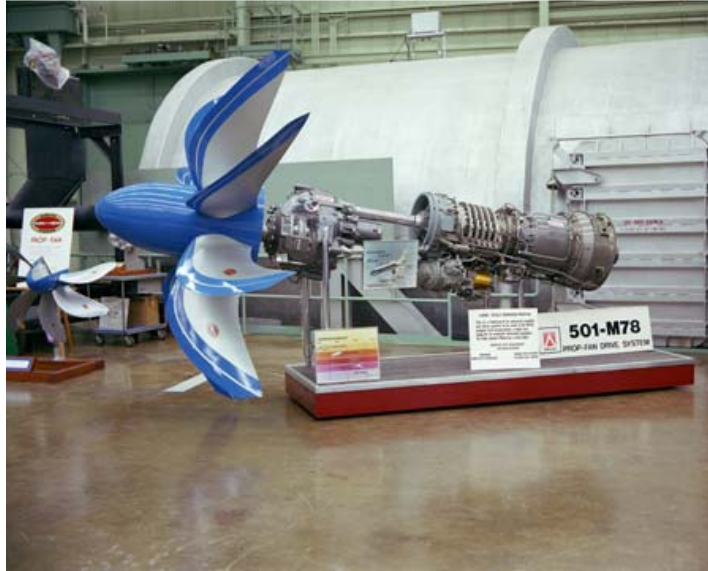
Figure 2-15 Allison 501-M78 Advanced Turboprop on display at NASA PSL [19].
