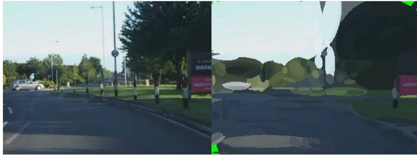
Figure 4.4: The MSCR feature detection algorithm input and output
