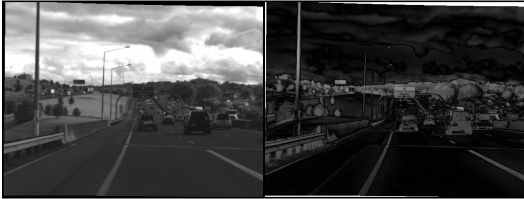
Figure 3.4: Difference of Gaussians using a 5-level pyramid with a 5 \times 5 Gaussian filter.
