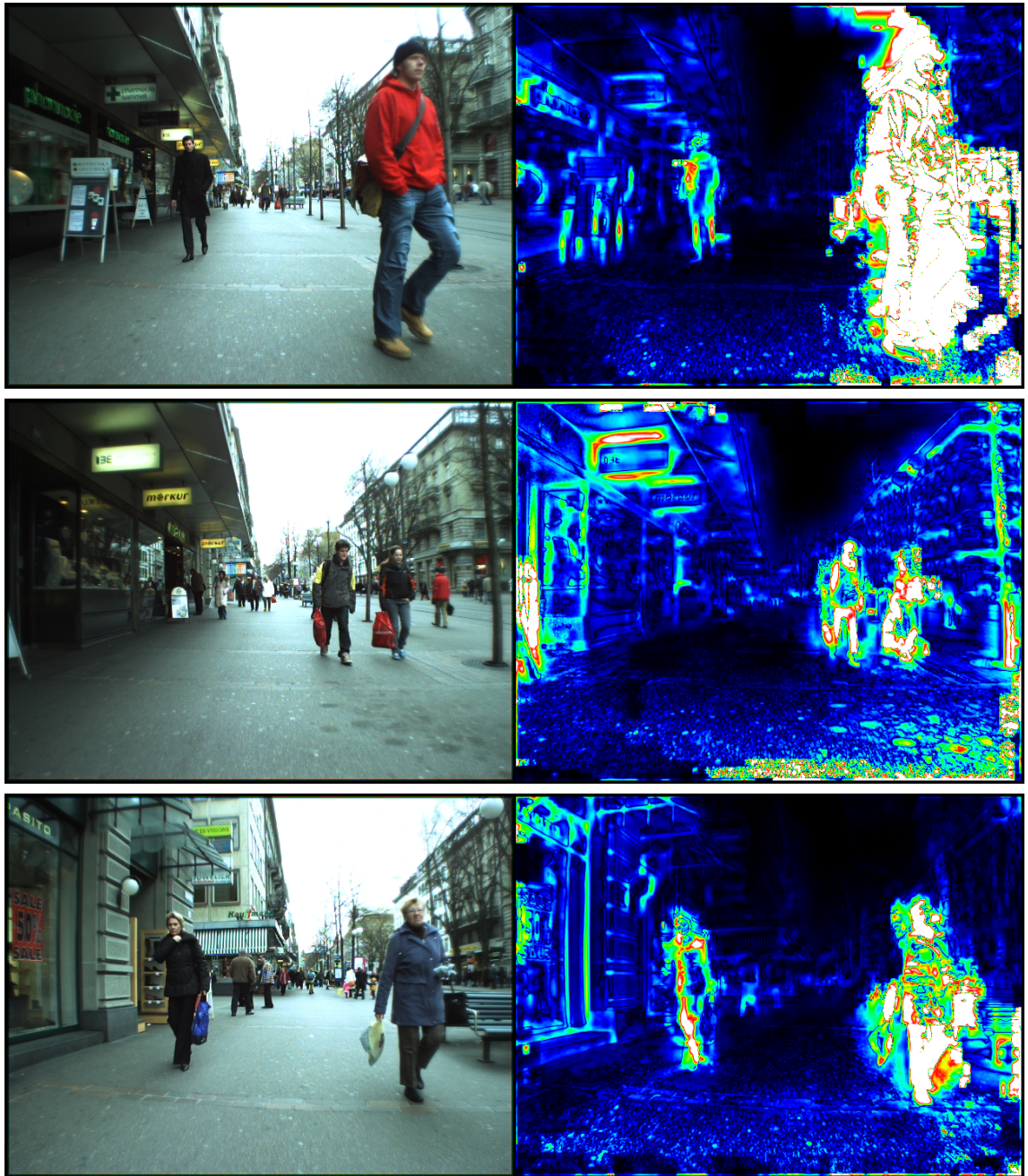
Figure 5.13: Fusion of DVoG saliency and DeGraF depth information in order to accelerate pedestrian detection. (ETH Dataset [12])
