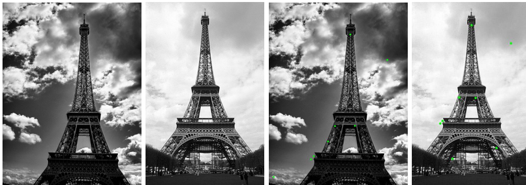
Figure 2.2: Two pictures of Eiffel Tower (left pair), taken under two different perspectives. A good feature detector must find those characteristic points that are distinctly recognisable in both images (right pair). A good feature extractor should define norms with invariant metrics in projective transformations.
