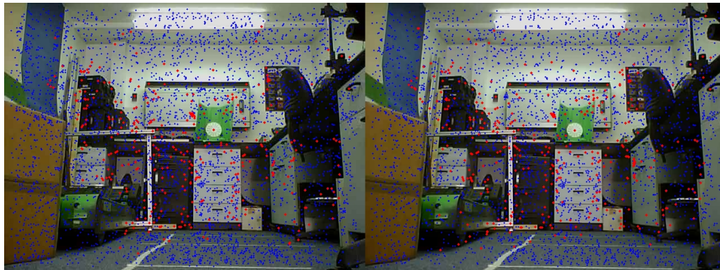
Figure 3.8: Effect of bilateral filtering over feature detection. The blue points are the initial feature points detected and the red points are the feature points that pass the filters in the matching stage. The feature detector used here is SURF (Bay et al. (2006)). 4927 feature points are initially detected in the raw image (left), whereas only 4328 are detected in the filtered image (right). However, only 354 go through the matching selection process in the raw image and 382 in the filtered image.
