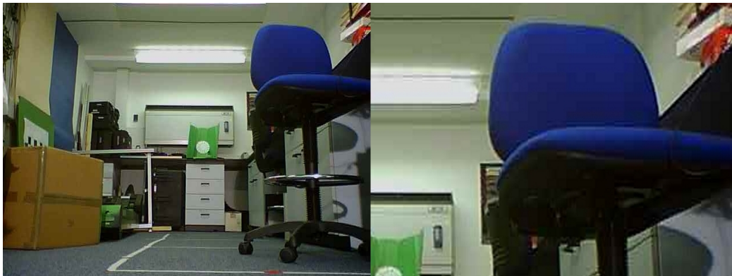
Figure 3.5: Mosquito effect in an image from the platform. On the zoomed in left-side photo the mosquito effect is noticeable around the edge of the chair and boxes.
