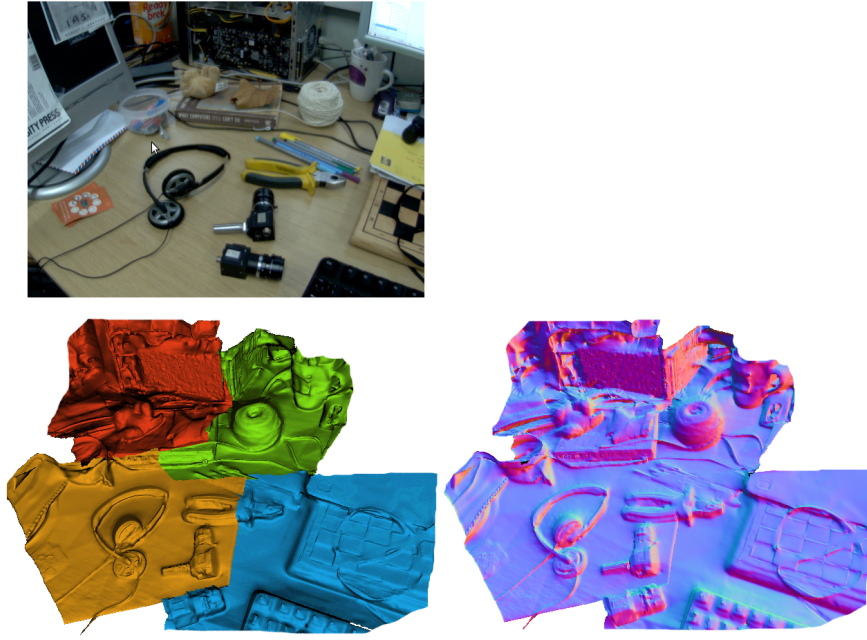
Figure 1.3: Dense reconstruction by Newcombe et al. (2011). Top: Overview of the scene. Bottom Left: four patch local 3D maps stitched into the global reference. Right: the final reconstruction.
