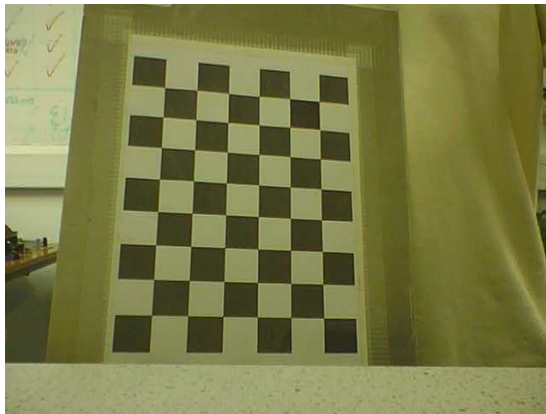
Figure 3.6: Checkerboard “Tsai grid” used for camera calibration.
