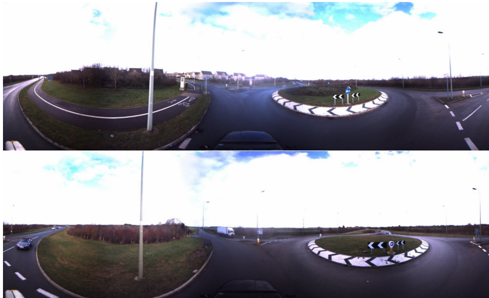
Figure 4.4: A false loop-closure assigned by FAB-MAP, described in Section 4.2.2. Source: Cummins and Newman (2011).
