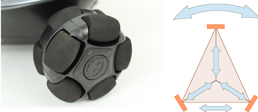
Figure 1.6: Left: omni-wheel detail; Right: possible motion directions for the omnidirectional robot platform.
