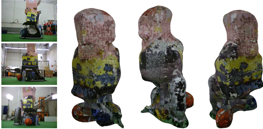
Figure 5.12: 3D surface of the object placed in the centre around which the platform in turntable sequence revolves.
