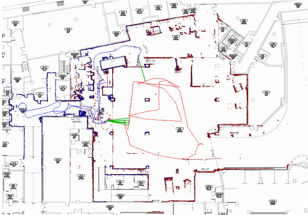
Figure 4.1: 2D mapping from direct encounters between a wheeled robot and a quadrotor. In blue the 2D map created by the wheeled robot, in red the 2D map created by the quadrotor. The green lines show where the encounters occurred. This result is from Kim et al. (2010).
