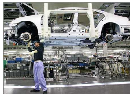
Car body on the conveyor line with wheel hubs installed (Turpen, 2012)
