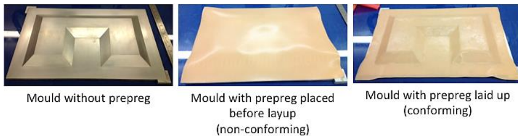
Figure 90: Workpiece progress from blank mould to fully laid prepreg
