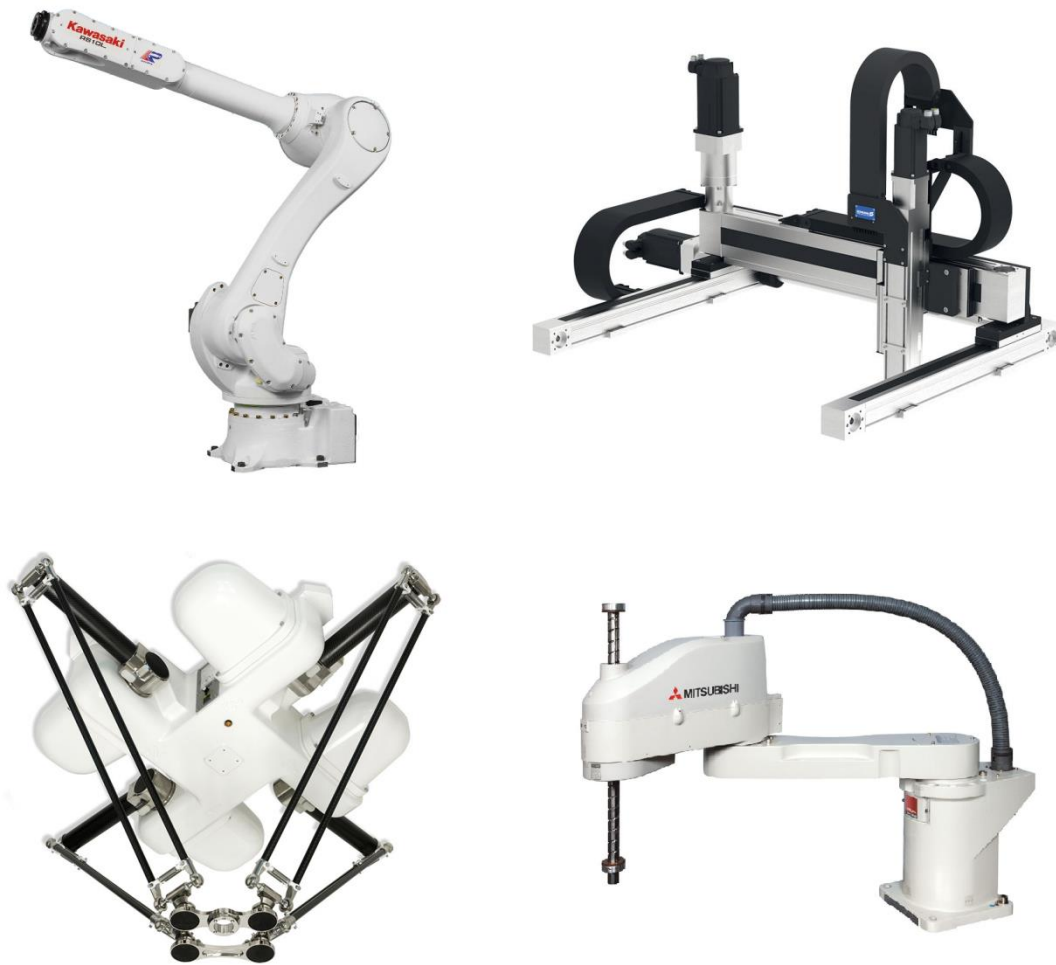
Figure 2-2 - articulated robot (top left); parallel robot (bottom left); Cartesian robot (top right); SCARA robot (bottom right)
