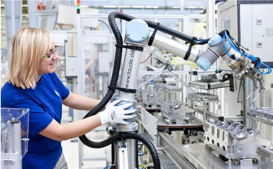
Figure 2-9 - industrial collaborative robot carrying out glow plug installation
