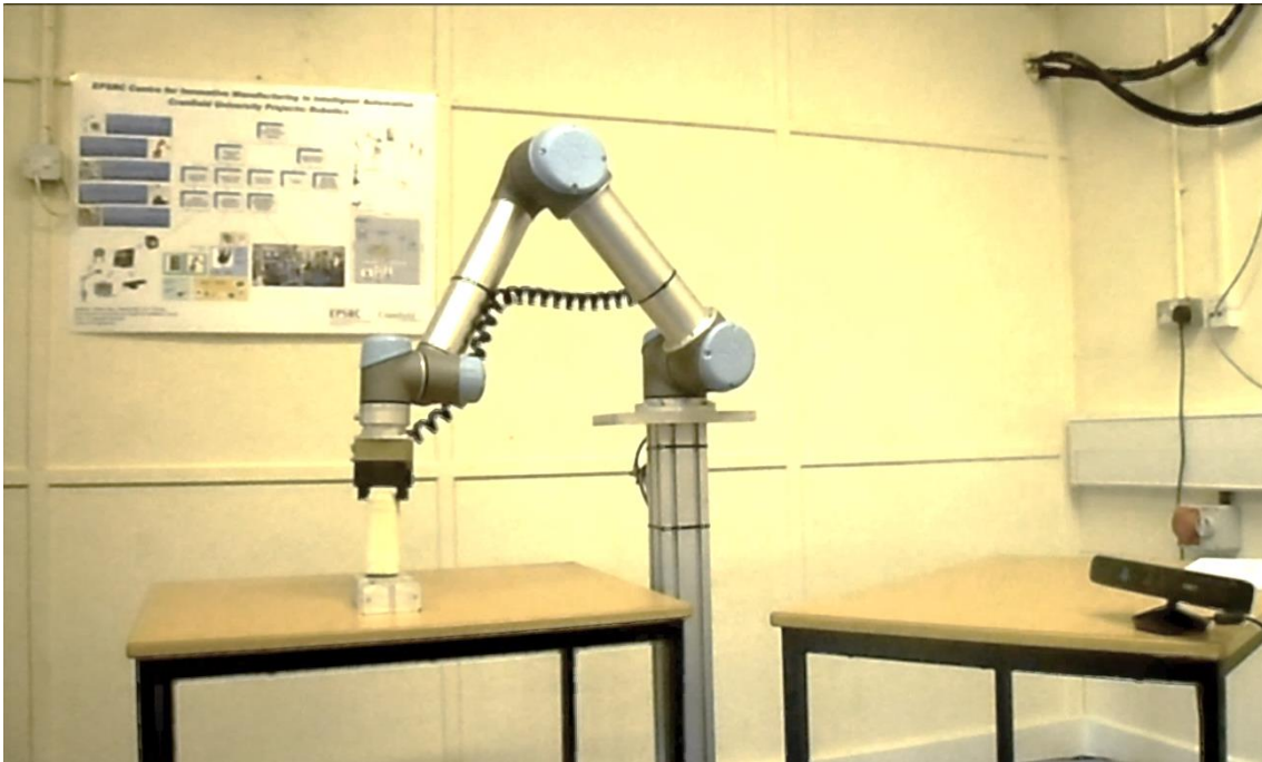
Figure 4-4 - Peg-In-Hole test using Virtual Directional Pad
