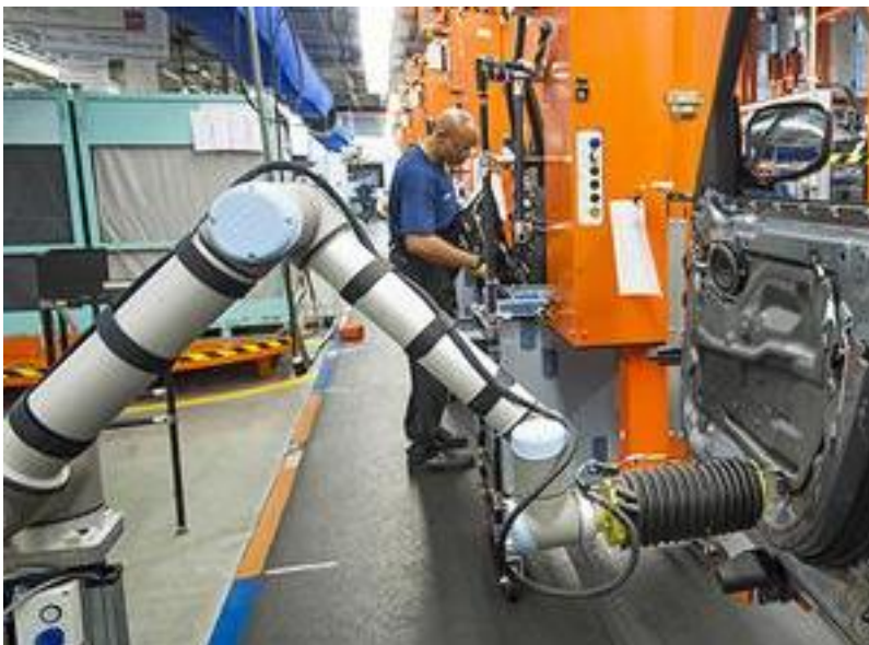
Figure 2-8 - industrial collaborative robot applying sealant on car door
