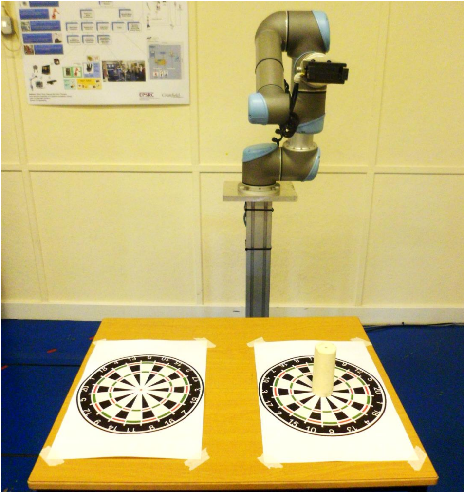
Figure 4-3 - pick and place test using Virtual Directional Pad
