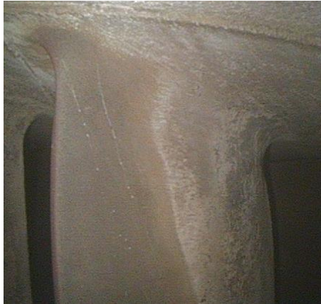
Figure 6-3: Blade with baked deposits
