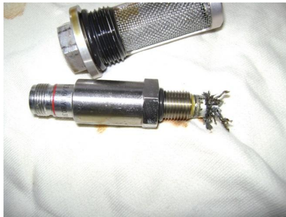
Figure 3-11: ECD and strainer with bearing debris
