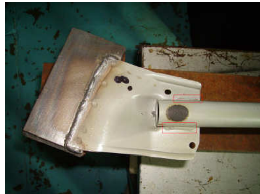
Fig. 8.7: welds between pipe and small bracket
