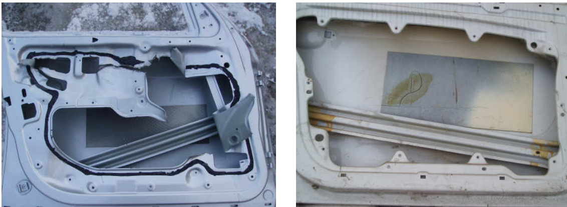
Fig.13.3: (on the left) Bmw X3 and Skoda (on the right) side-impact beams.
