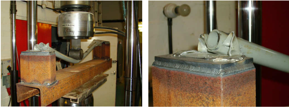
Fig. 9.8: beam under maximum load (left) and detail of the small bracket (right) when the test was stopped.
