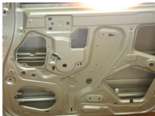
Fig. 8.8 side-impact-beam within the front door of Nissan Pathfinder / Navara.
