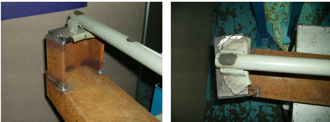
Fig. 9.9: details of the small bracket at the beginning of the bending test
