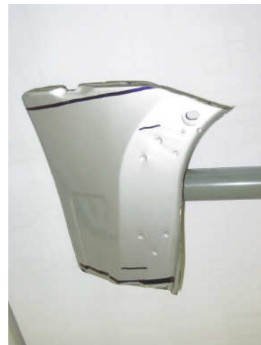
Fig. 8.11: position of spot-welds between the small bracket and the inner-skin of the door.
