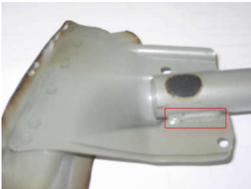
Fig. 8.7: welds between pipe and small bracket
