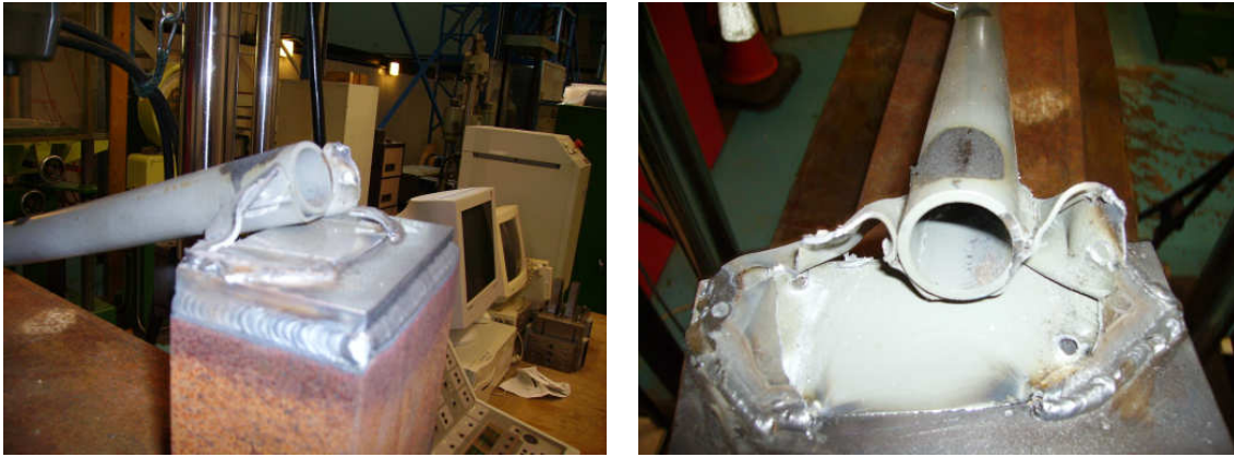
Fig. 9.10: details of the small bracket at the end of the bending test
