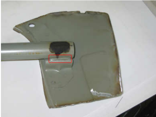
Fig. 8.6: welds between pipe and small bracket
