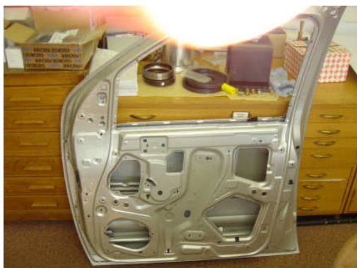
Fig. 8.8 side-impact-beam within the front door of Nissan Pathfinder / Navara.
