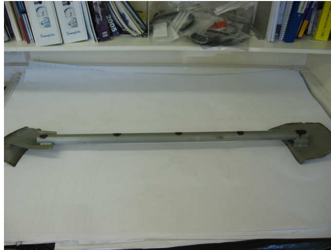
Fig. 8.12: position of the absorbers between the pipe of the side-impact-beam and the outer-skin of the door.
