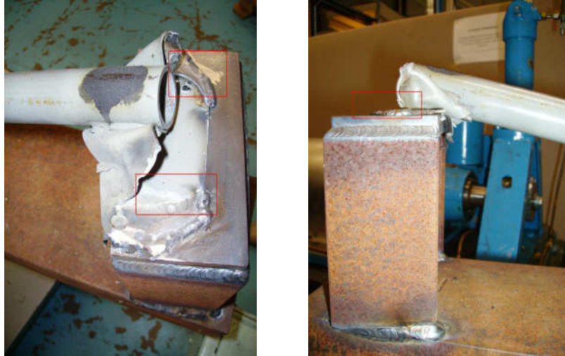
Fig. 12.1: tearing of material at the basis of the small-bracket.
