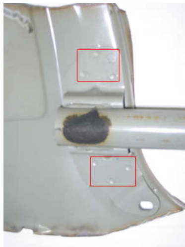
Fig. 8.11: position of spot-welds between the small bracket and the inner-skin of the door.
