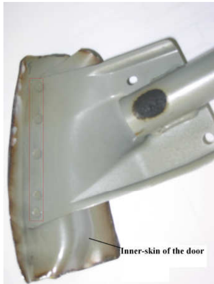
Fig. 8.10: position of the spot-welds between the big bracket and the inner-skin of the door.
