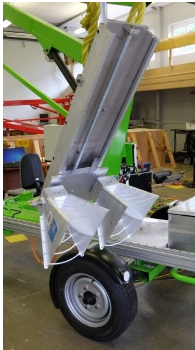
Fig. 1 Radar Interferometry mount repurposed for the collection of accurately aligned 2D apertures for 3D SAR image formation. The broadband horn antennas were mounted on the interferometer hand-wound mechanism.
